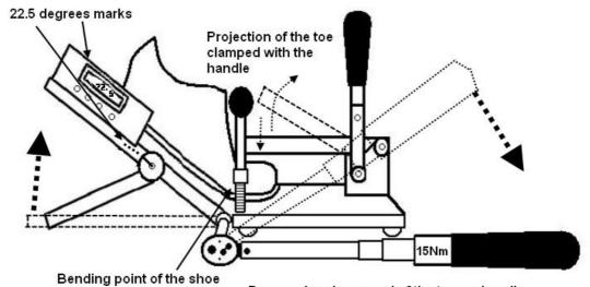
By pressing downward of the torque handle the platform will move up, the angle achieved before the torque wrench clicks or breaks, this indicates 15Nm of pressure has been achieved.
