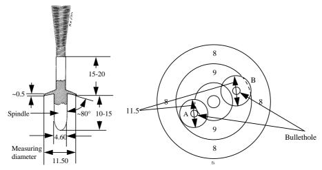
The "A" illustration depicts a doubtful shot hole with the outward scoring gauge in place. The outside edge of the flange is within the 9 ring; therefore the shot is scored a 10.
