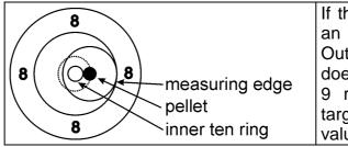
If the measuring edge of an Air Pistol Inner Ten Outward scoring gauge does not go outside the 9 ring of an air pistol target then the shot value is an inner ten.
