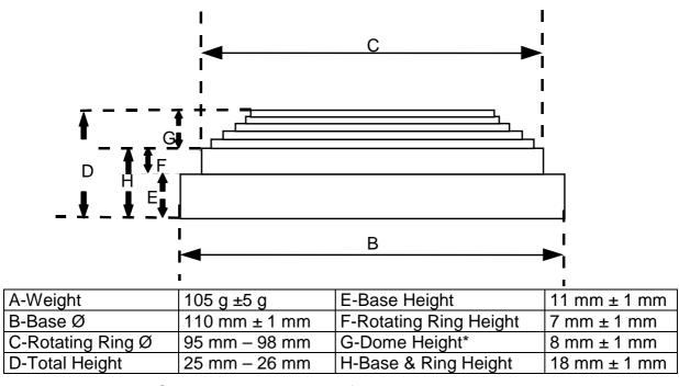
"G" - The actual shape of the target dome is to be engineered to provide the best aerodynamic design and flight stability.
